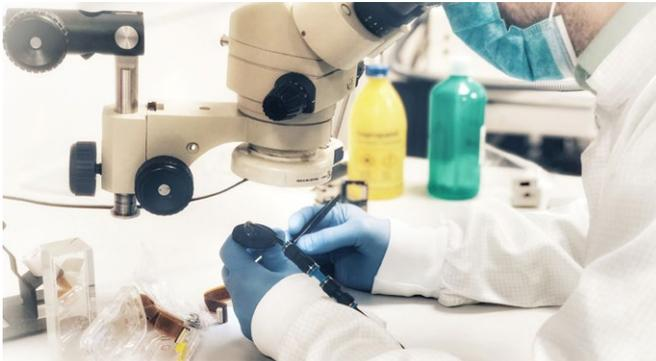
Fig. 1: Manual workstation with tweezers and microscope
